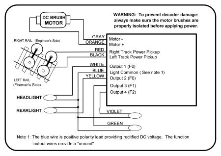
We recommend that the first full power testing be done on regular DC. If the track pickup polarity (red and black wires) is reversed you will want to correct this for proper analog mode operation. The decoders should be driven by a good quality <a href="mailto:smooth">smooth</a> DC power unit. Power packs with pulse power systems such as "tracking control", etc. will give unpredictable operation.
