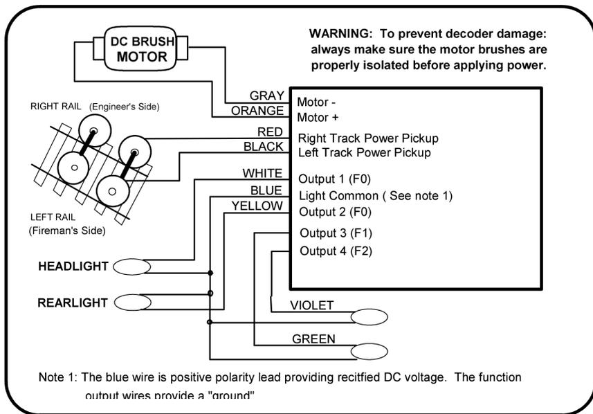
We recommend that the first full power testing be done on regular DC. If the track pickup polarity (red and black wires) is reversed you will want to correct this for proper analog mode operation. The decoders should be driven by a good quality smooth DC power unit. Power packs with pulse power systems such as "tracking control", etc. will give unpredictable operation.
