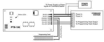
22 VDC. Minimum input voltage for reliable operation is 12 VAC or 14 VDC. Optionally, you may purchase and use a dedicated power supply rated at 15 volts DC, 500mA.
