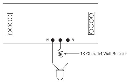
This MUST be a 3 leg Bi-Color LED with a Common Anode
