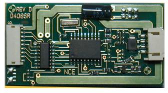
Dimensions:  $1.2 \times 2.30 \times ...375$  inches  $31 \times 59 \times 9.5$  mm Decoder version 3.5
