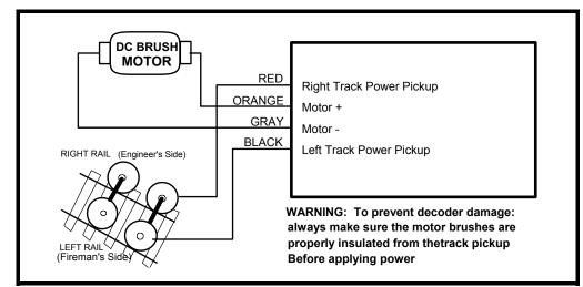
Before test running your newly converted locomotive on full power double check your wiring to make sure the motor is fully isolated and that there are no pinched or broken wires. We see many decoders returned due to wires getting pinched between the body shell and frame causing shorts. Always test your decoder installation on an current limited programming track <u>before</u> trying it on full track power.
