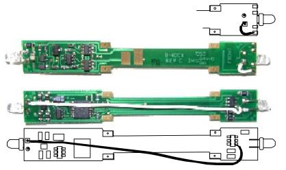
For Outputs 1 and 3, connect a short jumper from the square LED connection of the headlight to the #3 solder pad of the bottom side of the PC board.
