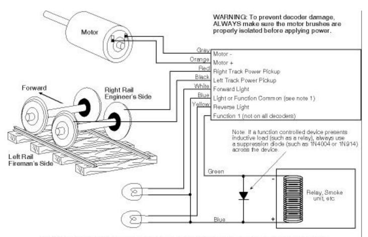
Note 1: The function common (blue wire) is the positive lead providing rectified DC voltage. If you elect to NOT use the common, power the light or other device from either track power pickup for "half-wave" operation (approx. 1/2 voltage).
