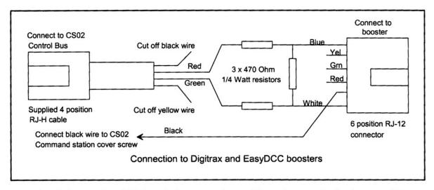
Note: With Digitrax or EasyDCC installations you only need the resistors to the first booster. You can then 'daisy chain' from booster to booster. The resistors are only needed to ensure that the mainline shuts down when the programming track is in use, otherwise programming commands will be sent to the boosters programming all locos on the mainline. The resistors can be eliminated if you just want to do a quick hook up for testing purposes.
