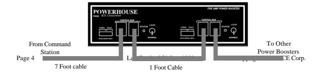
Use the supplied 7 foot cable to connect the PB-205a to your command station's CONTROL BUS socket. The remaining (unused) socket on the PB-205a cab be used to connect to other Boosters in daisy chain fashion. Use only the 4-wire RJ-H cable for this purpose. Longer cables may be used if more distance is needed between power stations. The last power station at the end of the daisy chain will have one empty socket. Each booster in the PB-205a will place a nominal 10mA load on the command station.
