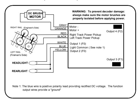
Before test running your newly converted locomotive on full power double check your wiring to make sure the motor is fully insulated from the frame and that there are no pinched or broken wires. We see many decoders returned due to wires getting pinched between the body shell and frame causing shorts.
