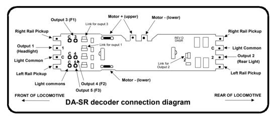
Always test your decoder installation on a current limited programming track <u>before</u> trying it on full track power.
