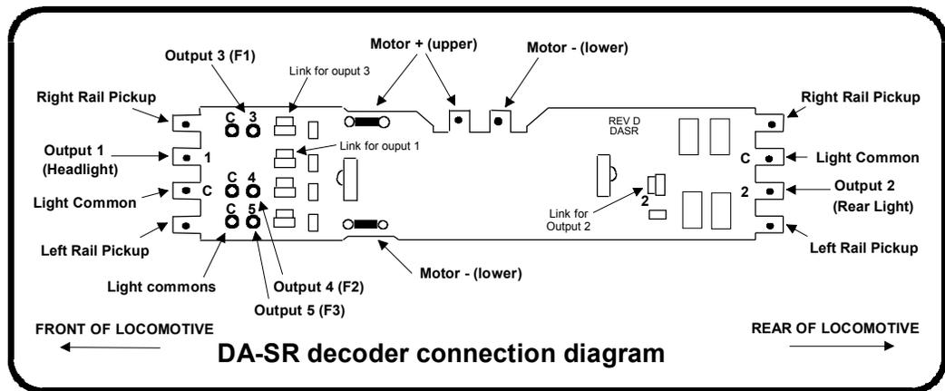
Always test your decoder installation on a current limited programming track before trying it on full track power.
