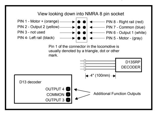
Plug the decoder in to the socket on the locomotive noting the pin 1 location. If you plug it in backwards no harm will be done but the locomotive will run backwards.
