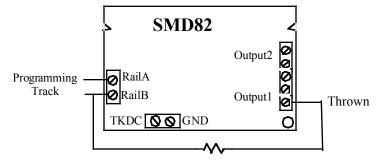
10 Ohm Resistor 1/2 Watt
