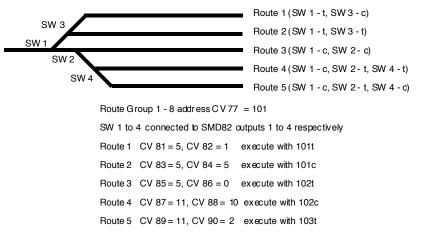
One SMD82 can handle routes with up to eight switches. However, it may be necessary to have routes with more than eight switches and consequently more than one SMD82. Multiple SMD82 can be programmed to operate together to execute a route with one command. Lets say you have a route with 16 switches. This would require two SMD82s.
