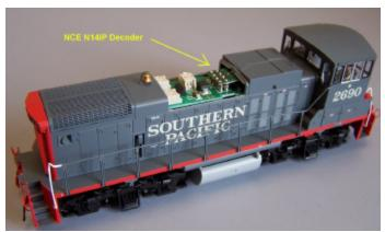
Limited space above the decoder plug in this locomotive presents a challenge for fitting a decoder. The NCE N14IP decoder is a good fit for this limited space. A small tab on the exhaust stack insert of the body shell protrudes inside the shell and keeps the shell from fully seating down on the decoder (see illustration directly below). A simple solution is to remove the lower portion of this tab on the rear of the stack insert (see circled areas in two smaller pictures farther below)
