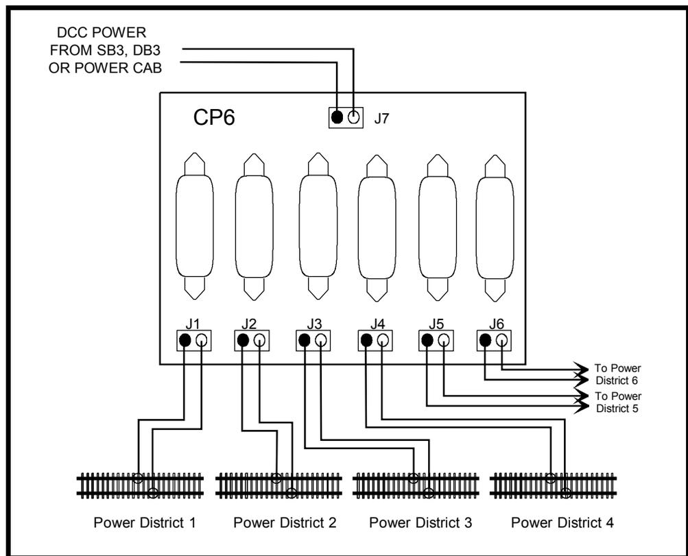
Note: The screw terminals marked with black dots in the drawing are connected together internally on the CP6 circuit board. If you are using common rail make sure the terminals marked in black above are connected to the common rail (bottom rail in the diagram).
