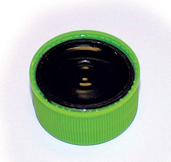
*Baffle Fabricated from Bottle Cap*
