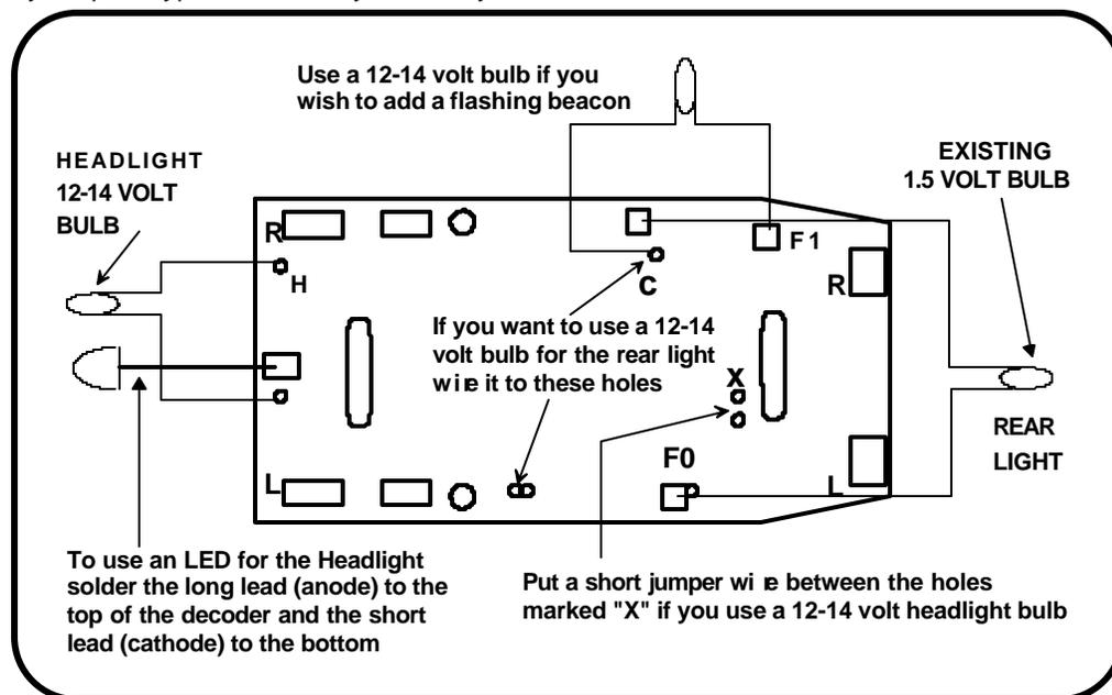
the holes marked "C" and "F1". The beacon is controlled by F1. The function is designed to use an incandescent bulb. (Miniaturics sells red bulbs) If you use a red LED an appropriate series resistor will also be required. The effect may not be as good with an LED.
