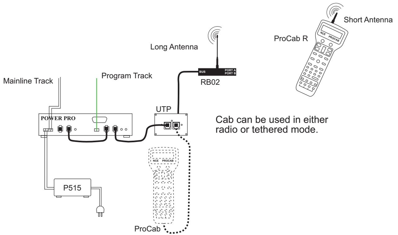
Cab can be used in either radio or tethered mode.
