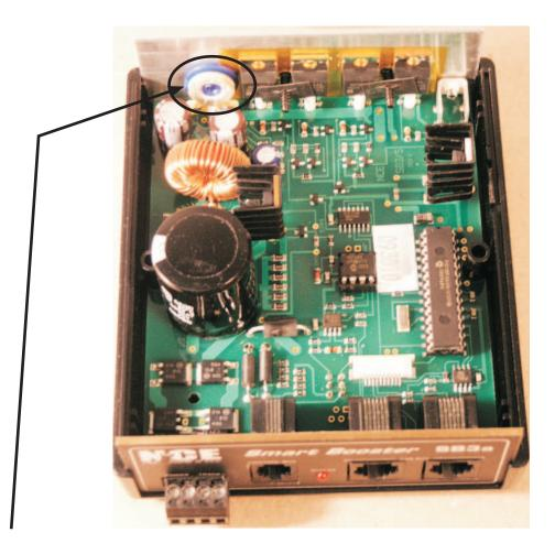
Turn this blue wheel and one way will increase the voltage, the other way will decrease. There is a hole on the back of the SB3a so you can get to it from the back with a small, flat screwdriver.
