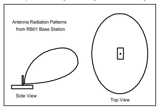
the antenna pointing down. See the diagram below for how the radio signal propagates from the antenna.
