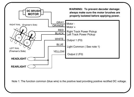
Before test running your newly converted locomotive on full power double check your wiring to make sure the motor is fully isolated and that there are no pinched or broken wires. We see many decoders returned due to wires getting pinched between the body shell and frame causing shorts.
