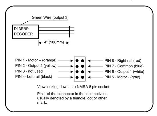
Plug the decoder in to the socket on the locomotive noting the pin 1 location. If you plug it in backwards no harm will be done but the locomotive will run backwards. Before test running your newly converted locomotive on full power double check your wiring to make sure the motor is fully isolated and that there are no pinched or broken wires. We see many decoders returned due to wires getting pinched between the body shell and frame causing shorts.
