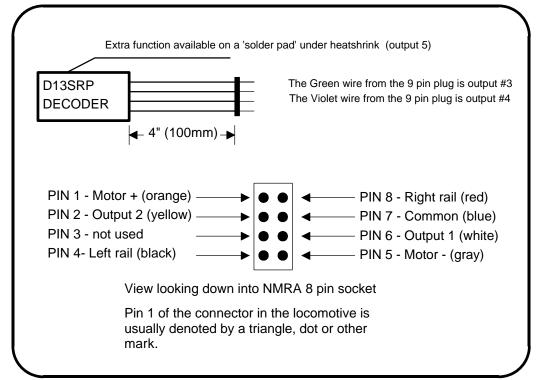
Before test running your newly converted locomotive on full power double check your wiring to make sure the motor is fully isolated and that there are no pinched or broken wires. We see many decoders returned due to wires getting pinched between the body shell and frame causing shorts.
