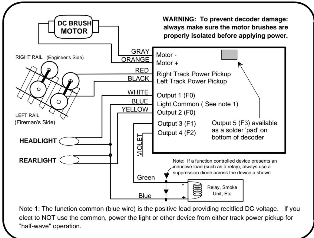
Before test running your newly converted locomotive on full power double check your wiring to make sure the motor is fully isolated and that there are no pinched or broken wires. We see many decoders returned due to wires getting pinched between the body shell and frame causing shorts.
