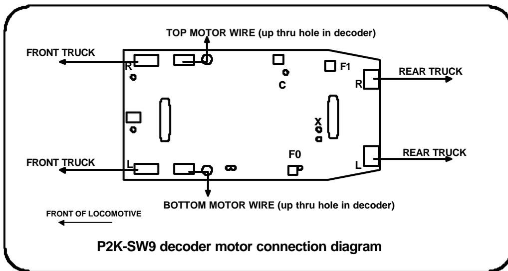
Now is a good time to test the locomotive before installing the lights and replacing the body shell. Double check your wiring and make sure that there are no pinched or broken wires. We see many decoders returned due to wires getting pinched between the body shell and frame causing shorts.
