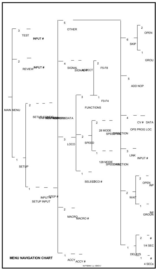
The following commands can be setup through the ProCab user interface and sent by the Mini Panel:
