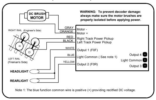
Before test running your newly converted locomotive on full power double check your wiring to make sure the motor is fully insulated from the frame and that there are no pinched or broken wires. We see many decoders returned due to wires getting pinched between the body shell and frame causing shorts.
