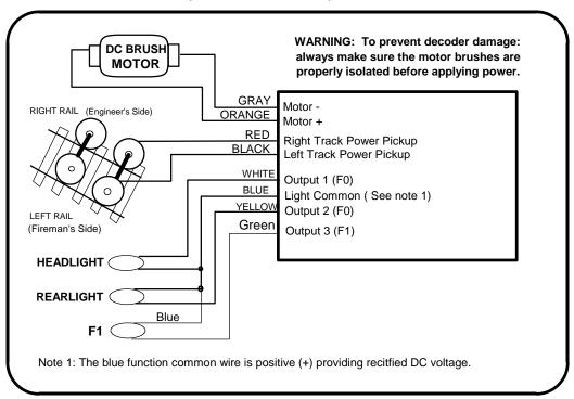
Before test running your newly converted locomotive on full power double check your wiring to make sure the motor is fully insulated from the frame and that there are no pinched or broken wires. We see many decoders returned due to wires getting pinched between the body shell and frame causing shorts.
