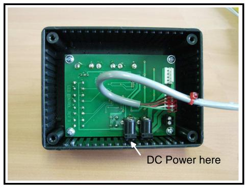
Put the controller box cover back on. Plug the power supply in to the topmost jack (indicated in the photo above) on the side of the contoller. Don't worry if you get the connections wrong, nothing will get hurt. One of the power supply jacks powers one of the white connectors the other power supply jack powers the other white connector.
