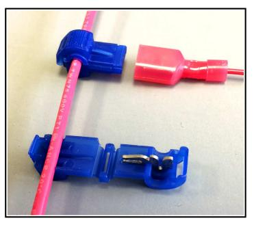
Fold the other half of the tap over on itself and crimp the tap closed with a standard pair of pliers as shown iin the photo to the right. Be sure to squeeze until you hear the tap 'click' together. Do not re-use a tap that has been damaged due to mis-crimping.
