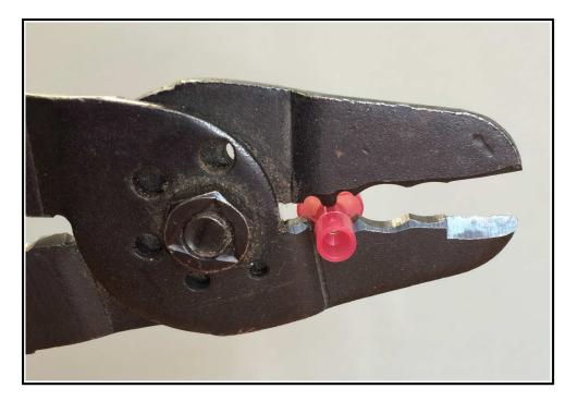
Squeeze the crimper sufficiently hard to dimple the insulation of the connector deeply without destroying the plastic covering. When done test the integrity of your crimp by trying to pull the wire back out of the connector. If it comes out you didn't use enough pressure.
