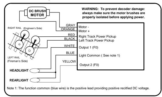
Before test running your newly converted locomotive on full power double check your wiring to make sure there are no pinched or broken wires. We see many decoders returned due to wires getting pinched between the body shell and frame causing shorts.
