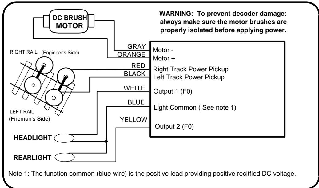
Before test running your newly converted locomotive on full power double check your wiring to make sure there are no pinched or broken wires. We see many decoders returned due to wires getting pinched between the body shell and frame causing shorts.
