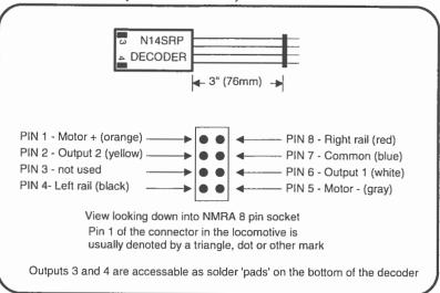
Before test running your newly converted locomotive on full power double check your wiring to make sure the motor is fully insulated from the frame and that there are no pinched or broken wires. We see many decoders returned due to wires getting pinched between the body shell and frame causing shorts.
