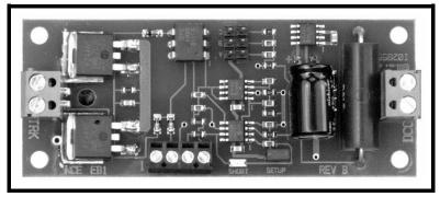
Electronic circuit breaker for use on DCC layouts only.
