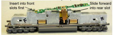
Step 5: Test the locomotive before replacing the body shell.
