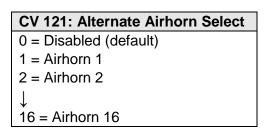
Remember, you can activate the alternate airhorn with the long airhorn function *only* when the short airhorn function is turned on. Set CV 121 to a value from 1 to 42 to select the alternate airhorn; the alternate airhorn is disabled when CV 121 is set to a value of 0.
