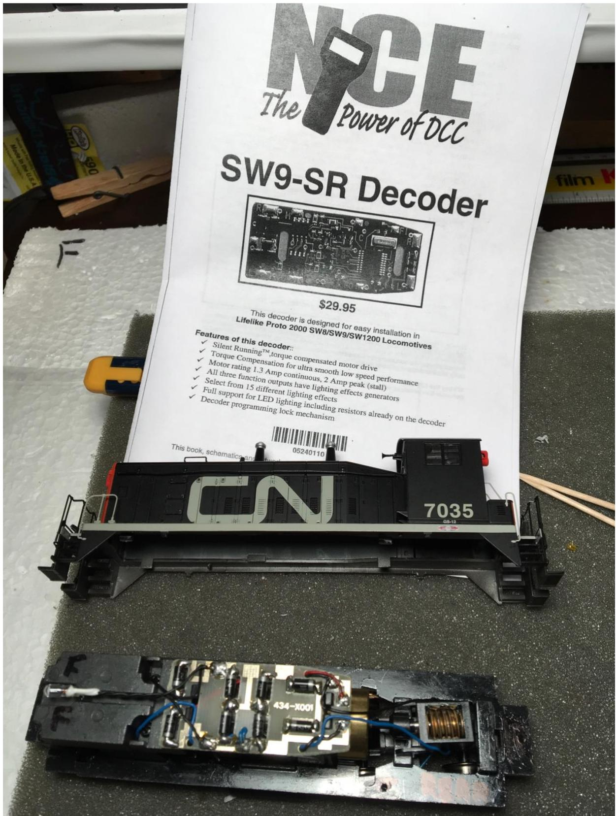
**Install an NCE SW9-SR mobile Decoder into an P2K SW1500 switcher.** Page 2 of 14
