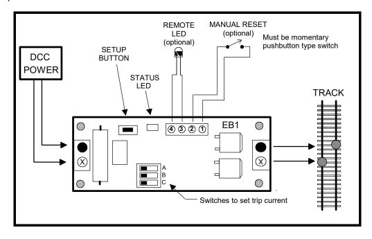
Note: The screw terminals marked with black dots (drawing above) are directly connected together on the EB1 circuit board. If you are using common rail make sure the terminals marked in black above are connected to the common rail (left rail in the diagram). When the EB1 "trips" only the screw terminals marked with an X are disconnected during a short circuit.
