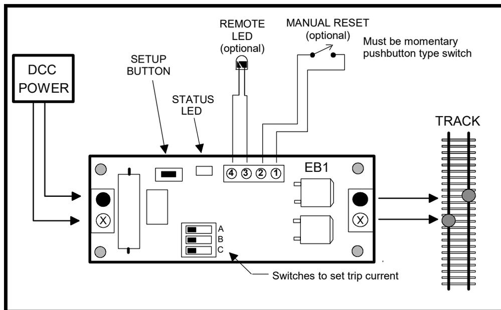
Note: The screw terminals marked with black dots (drawing above) are directly connected together on the EB1 circuit board. If you are using common rail make sure the terminals marked in black above are connected to the common rail (left rail in the diagram). When the EB1 “trips” only the screw terminals marked with an X are disconnected during a short circuit.
