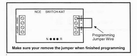
To set the "ON TIME" of the decoder outputs (factory default is 40 milliseconds)
