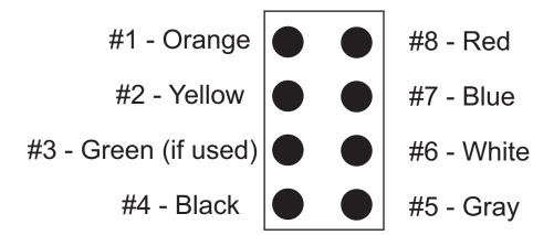
View is looking down on the wires. The 'pins' are on the other side.
