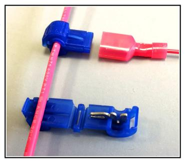
Fold the other half of the tap over on itself and crimp the tap closed with a standard pair of pliers as shown iin the photo to the right. Be sure to squeeze until you hear the tap 'click' together. Do not re-use a tap that has been damaged due to mis-crimping.
