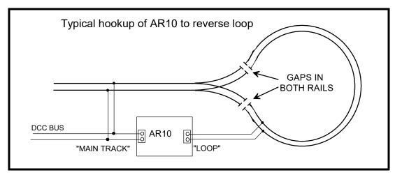
If you have a situation where the loop cannnot be made longer than your longest train you will need a second set of gaps in both rails creating a short dead section the length of the longest metal truck in the train. This will be required at both the entrance and exit of the loop.
